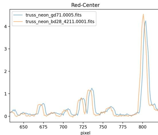
The same effect is seen for the internal lamps. The BD+284211 pointing seemed to have a significantly different grism position. However, the three other pointings appeared remarkably stable, despite numerous changes to the grism setup.
