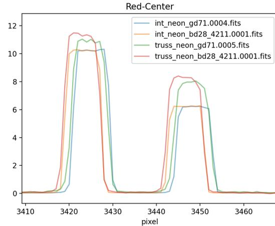
We can also pair the truss & internal lamps at the same pointings. Thankfully the internal and truss lamps seem to give fairly consistent solutions. I do note, however, the profiles of the internal arc lines are more flat-topped, even for small-amplitude lines (i.e. I don't believe this is a saturation issue). Could this indicate a scattered-light issue?
