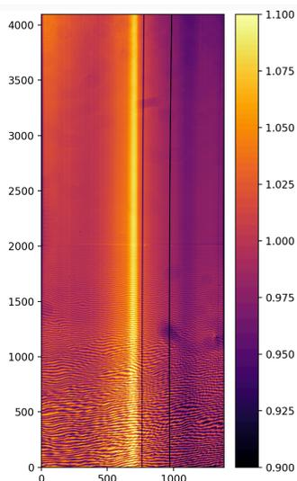
We did not test the internal versus truss quartz lamps for any other grism mode, but I do note a similar slit-like reflection feature is present in this example from co-adding 5 internal flats in the Red-Center mode.
