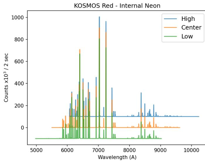
There is a nice region centered around 6100Å with ~4 strong Neon lines that is accessible at *all* grism configurations. Neon is therefore always a good bet for doing frequent wavelength calibrations (e.g. at every pointing).
