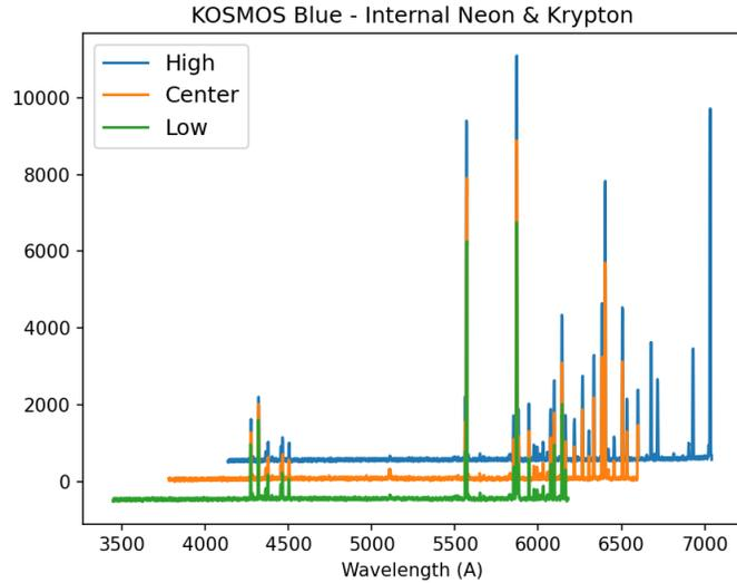
Even just using Neon and Krypton, reasonable wavelength solutions are possible for the entire blue range (above). These lamps should be taken at all blue positions as well. Overall KOSMOS reaches from ~3800 angstroms to around 1micron. Red-Low is an excellent default position using NeKr for wavelength calibration. I naively computed a mean spectral resolution *per pixel* of  $\lambda_p / \Delta\lambda_p \approx 7000$  in both red and blue modes.
