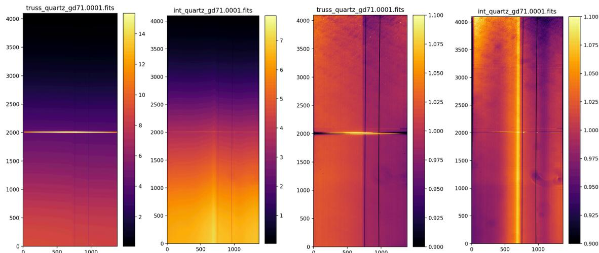
**Left:** flat field images for truss and internal lamps, normalized by the median value of the flat.
