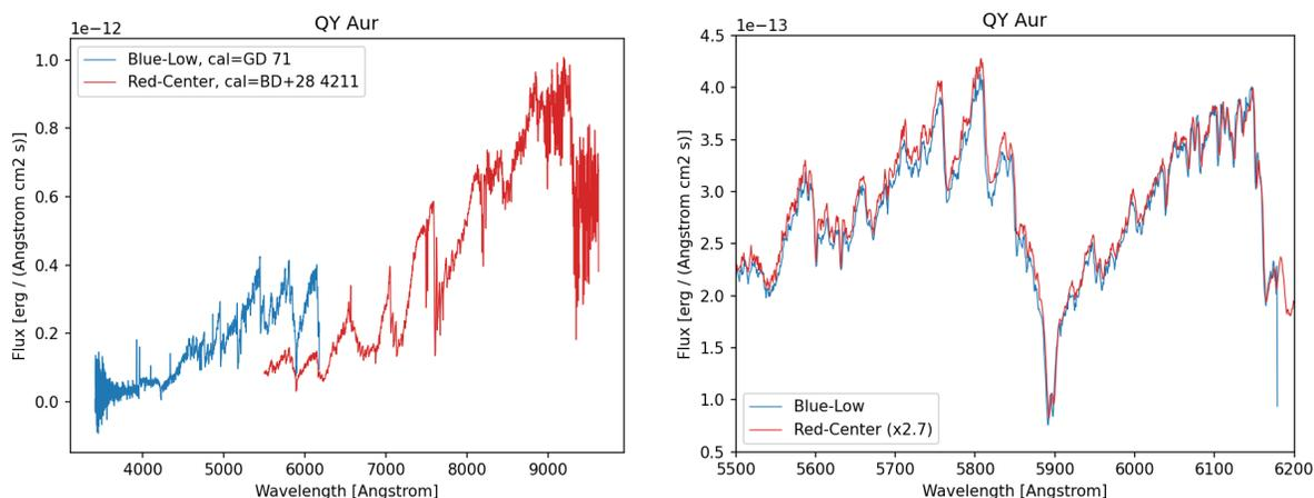
For completeness, I also fully reduced the Blue-Low data for BD+28 4211. Using the spec50cal IRAF data to generate the sensfunc for this target in both red and blue modes, the flux-calibrated spectrum below looks very reasonable.
