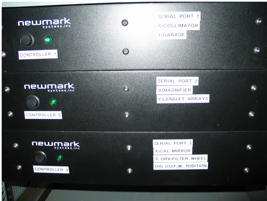
Fig. C5 Detail of Newmark controllers. Power switches are to the left, with green power indicator lights. Various drive components controlled by each Newmark are indicated to the right. The filter wheel controller is at the bottom of the stack.
