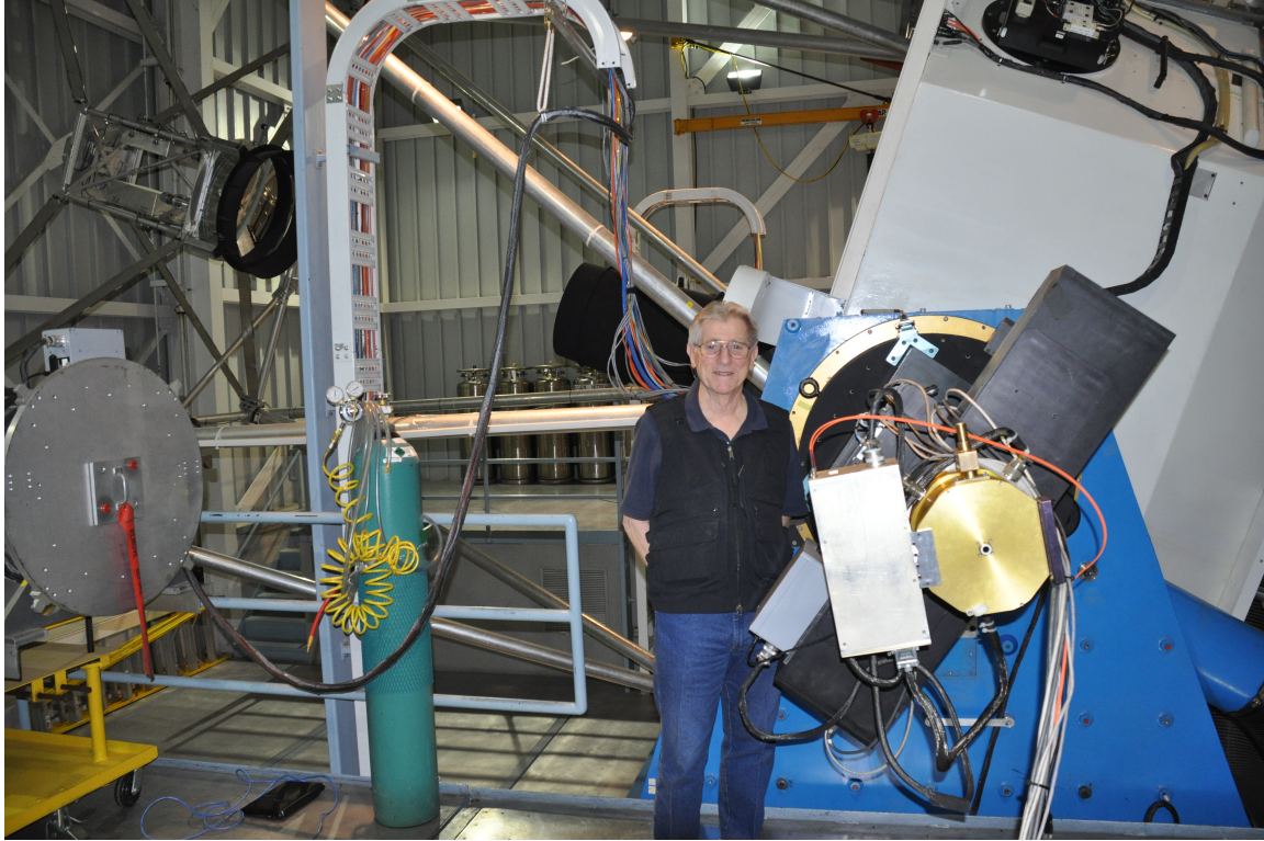
Fig. C.3 Back View of GIII mounted on the telescope. The gold circle is the GIII dewar. The silver rectangle to the left of it is the Leach controller. The disperser drive is the large, black rectangle.
