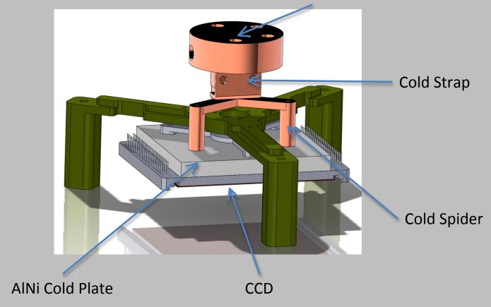
AlNi cold plate used as an electrical insulator while having good thermal conductance
