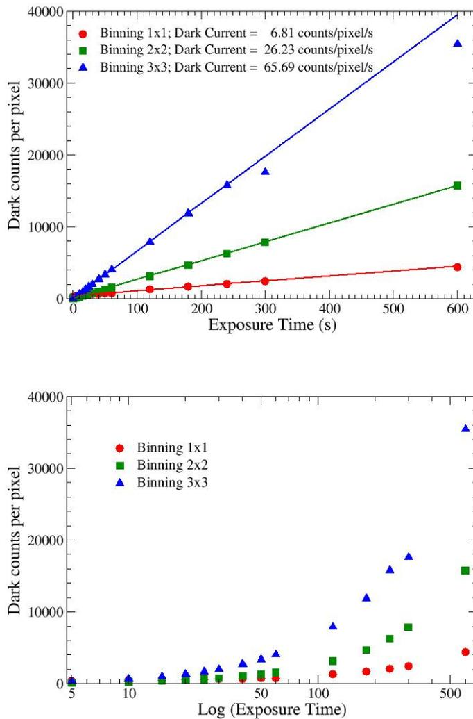
Figure 2: We show the dark counts obtained per pixel as a function of exposure time. With  $1 \times 1$  binning, we obtain a dark current of 6.8 counts/pixel/s. We expect to obtain  $n^2$  times as much dark current with  $n \times n$  binning and find that this expectation holds true within uncertainties for  $2 \times 2$  and  $3 \times 3$  binning.
