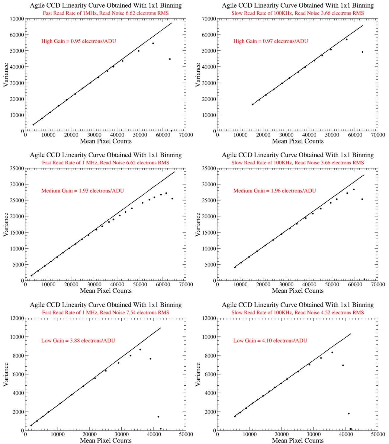
Figure 3: The CCD transfer curves show the linear regime of the CCD for each setting of read rate and gain. Please note that when binning 1x1 at the low gain setting, the CCD will saturate at about 43000 counts. However when binning 2x2, bear in mind that the saturation point should be given by the digitization limit of 65535 counts.
