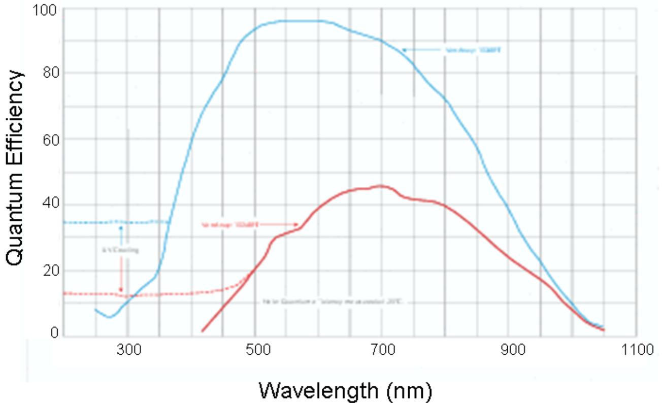
Figure 1: The solid and dotted blue curves indicate the Agile CCD quantum efficiency.
