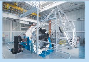
Beginning in 1991, the ARC 3.5-m Telescope's innovative software, mechanical, and optical designs provided users with high quality data and user-friendly operations. Light is collected by the 11.4-ft. spin-cast, glass, primary mirror and fed to any one of the multiple instruments mounted on the telescope. Observing programs are remotely conducted from locations around the globe by astronomers using the Internet and a unique software program.
