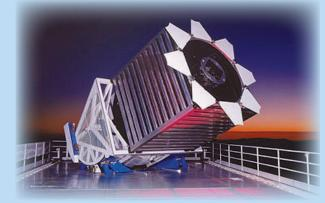
Operating since 1996, the Sloan Foundation 2.5-m Telescope conducts astronomical surveys using instruments to accurately measure distances and composition of celestial objects. A 2.5° imaging field or a 3° spectroscopic field is usable; light from these objects 'drifts' across the instrument as the Earth rotates. The telescope and instrument are exposed for observations at night when its enclosure building wheels away.
